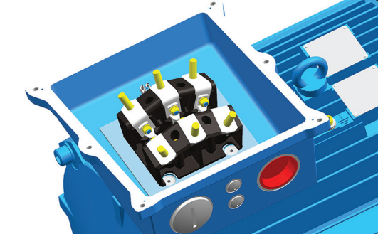
Terminal board for motor size 280 to 355.
