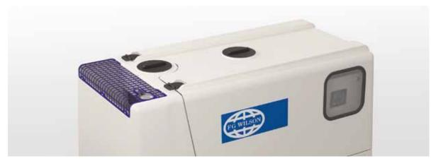
With a modern design, the two-component enclosure structure (hood and base), encompassing a sloped roof for optimal water run off, delivers enhanced water ingress protection. Raised access caps featuring compression seals, provide access points to the radiator fill and single point lift, while continuing to provide excellent protection against water ingress.
